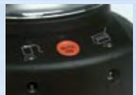
DC input from 12V solar module, mains adaptor or vehicle cigarette-lighter socket
